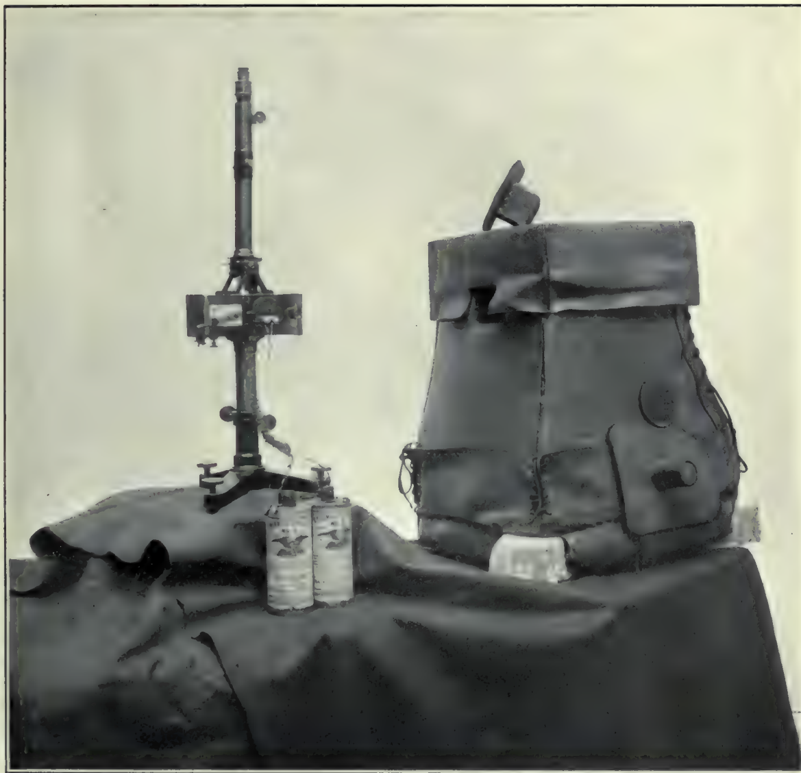
FIG. 3.—PRESENT PENDULUM APPARATUS SHOWING VERTICAL FORM OF TELESCOPE, ELECTRIC ILLUMINATION FOR OBSERVING SLIT, AND THE FELT-AND-LEATHER CASE FOR CONTROLLING THE TEMPERATURE.
